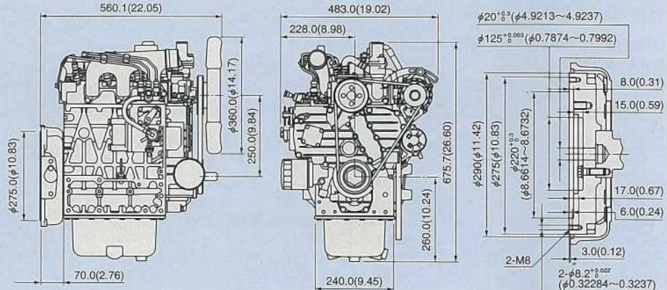
\*Various options (such as Shallow Oil Pan, Horizontal Water Outlet etc.) are available to reduce engine height.
