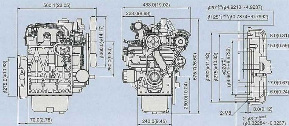
\*Various options (such as Shallow Oil Pan, Horizontal Water Outlet etc.) are available to reduce engine height.
